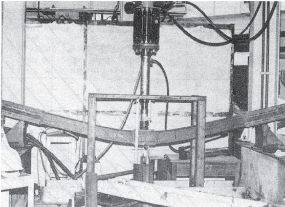
Plate 3. Steel hollow section under loading test
