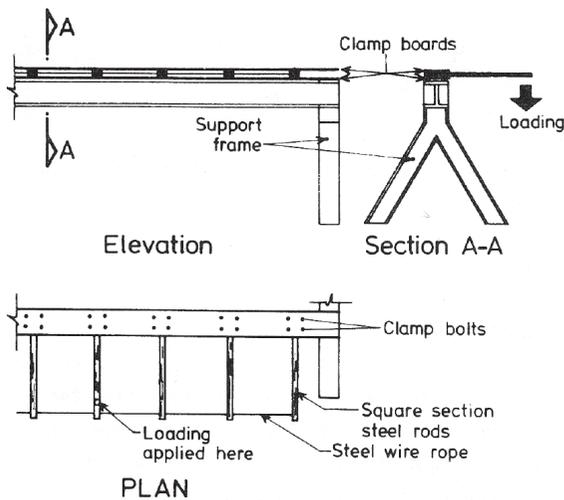
Figure 8. The set-up for experiment on fence-boulder interaction
