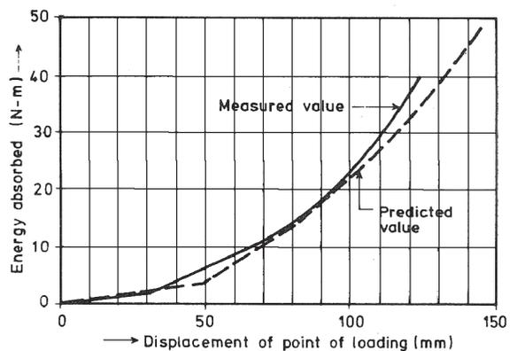
Figure 9. Energy absorption by model fence and its prediction by mathematical simulation
