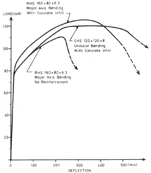
Figure 11. Test results on hollow sections
