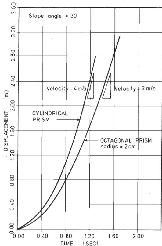
Figure 4. Typical time-displacement relationship for octagonal and cylindrical prisms
