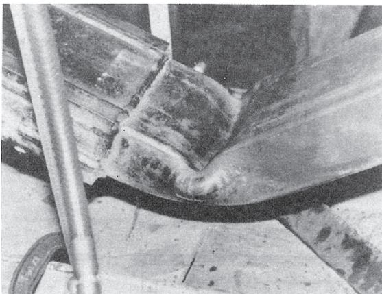
Plate 4. Local buckling of a rectangular hollow section
