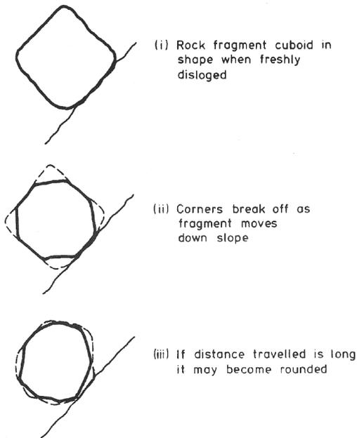
Figure 2. Development of shape of boulder down a slope
